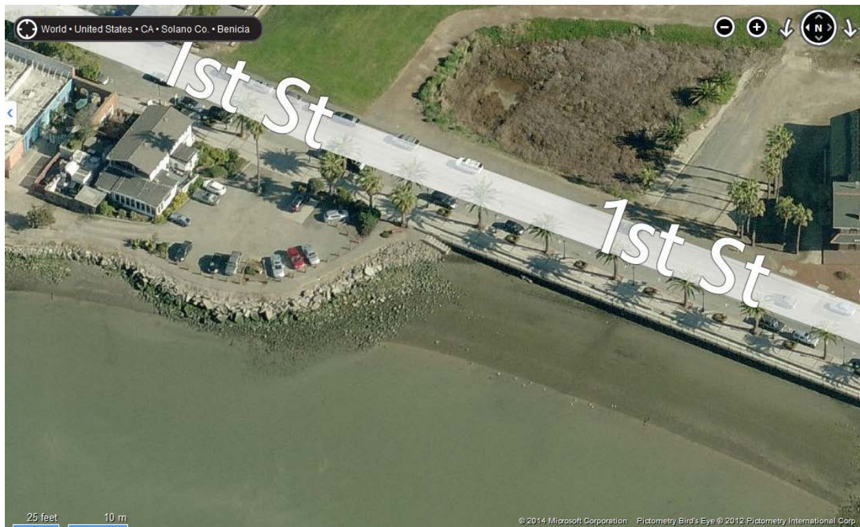
Figure 7: Non-engineered slope protection (left) and seawall (right)
