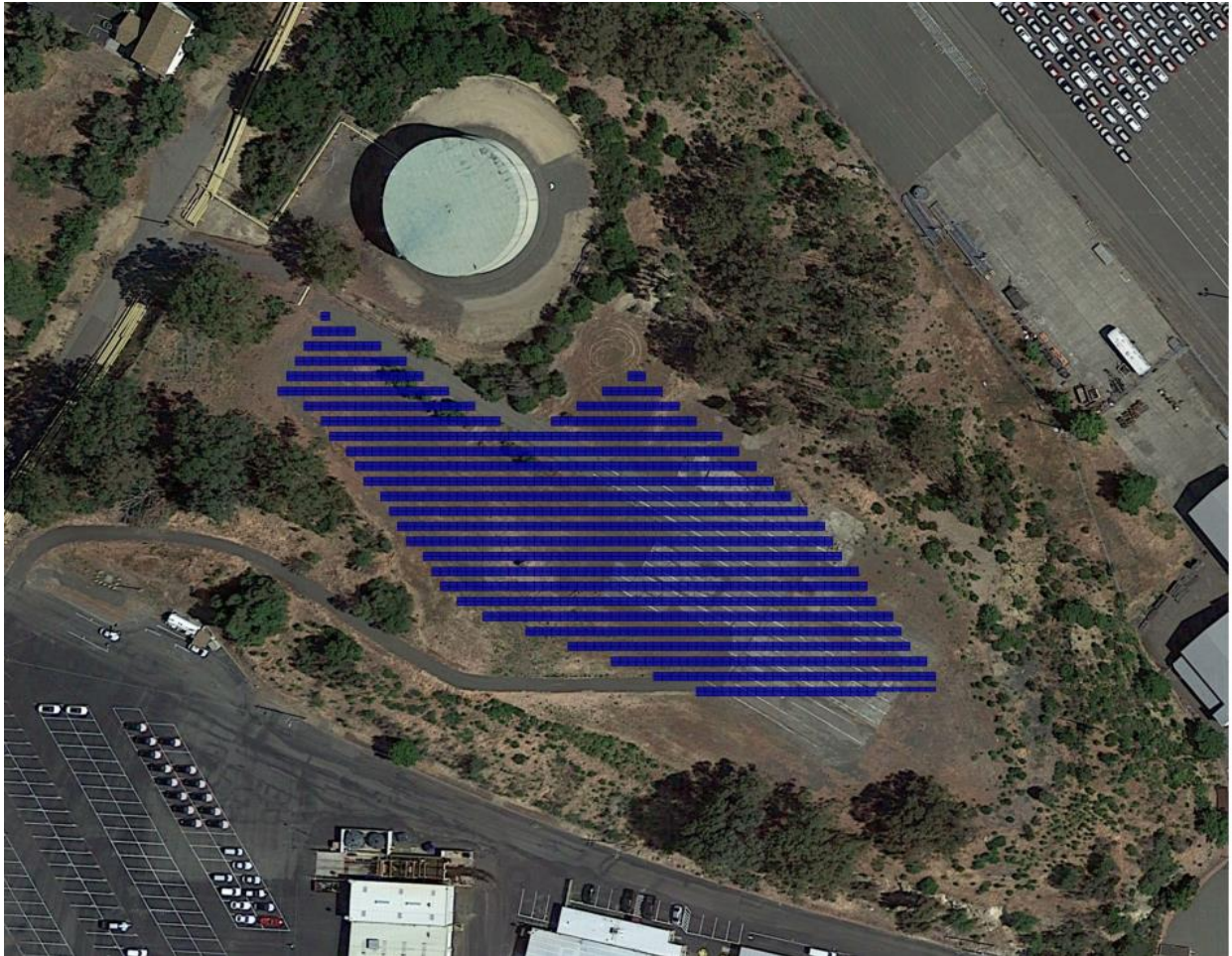
Figure 3. Amports site with 592 kW of photovoltaics.
