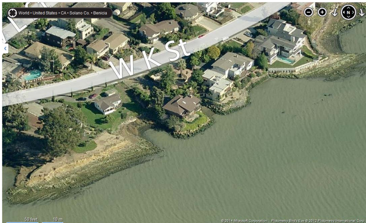
Figure 6: Unprotected bluff (left), engineered revetments (center), sea wall (right)
