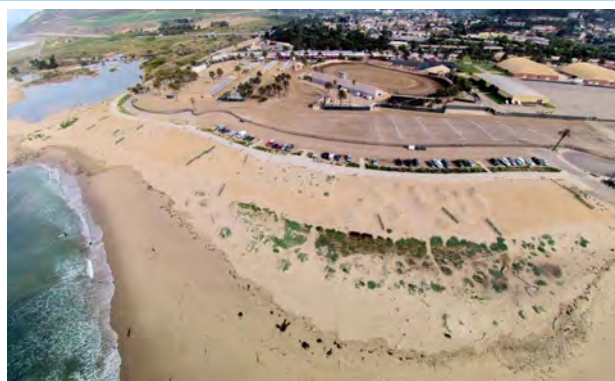
Example of managed retreat approach. Surfer's Point Managed Shoreline Retreat Project in Ventura, CA relocated the parking lot away from the shoreline and restored the beach area with cobbles and sand. Photo source: Surfrider Foundation 2013.
