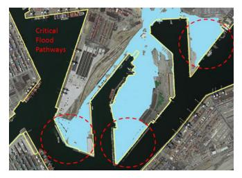
Figure 4-4. Example of critical flood pathways
